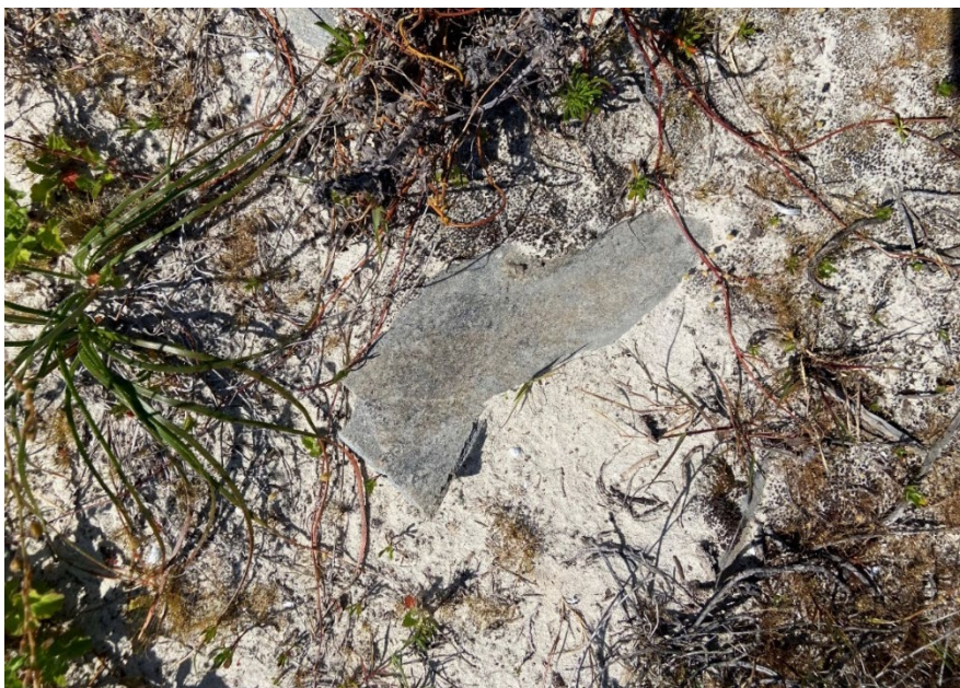
Plate 3-13: Potential Asbestos Containing Material
